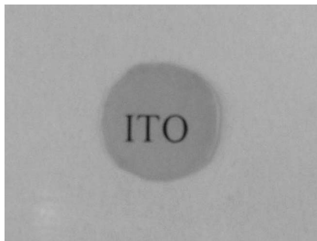
Fig. 4 Ink-jet printed and densified \text{In}_2\text{O}_3\text{:Sn} (ITO) layer with a thickness of 500 nm on paper. The letters 'ITO' printed on white paper illustrate the transparency of the \text{In}_2\text{O}_3\text{:Sn} layer.
